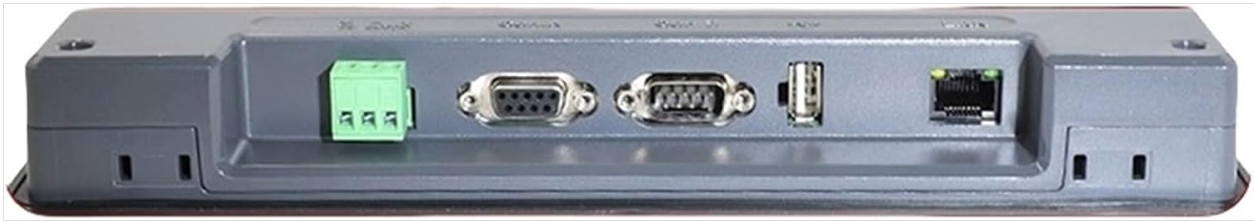
Figure 2: Rear view of the SHHJCO cMT-1107X HMI Touch Panel. This image highlights the various connectivity options, including a green terminal block for power input, two DB9 serial ports, a USB port, and an Ethernet port for network communication.
