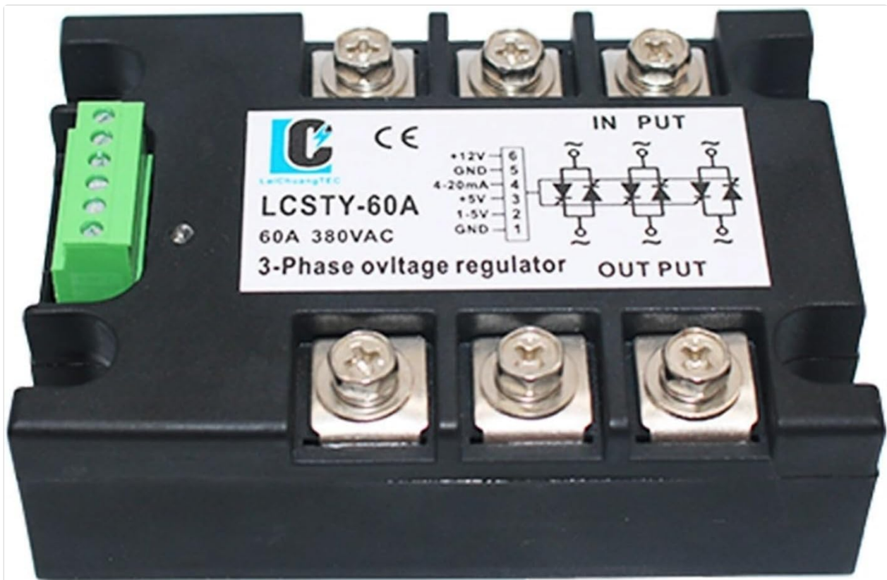
Figure 2: Angled view of the Voltage Regulator Module.
