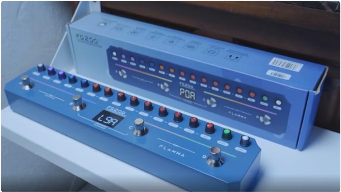
Figure 10: The FG200 pedal with the display showing tuner mode, activated by pressing and holding footswitches A and B.
