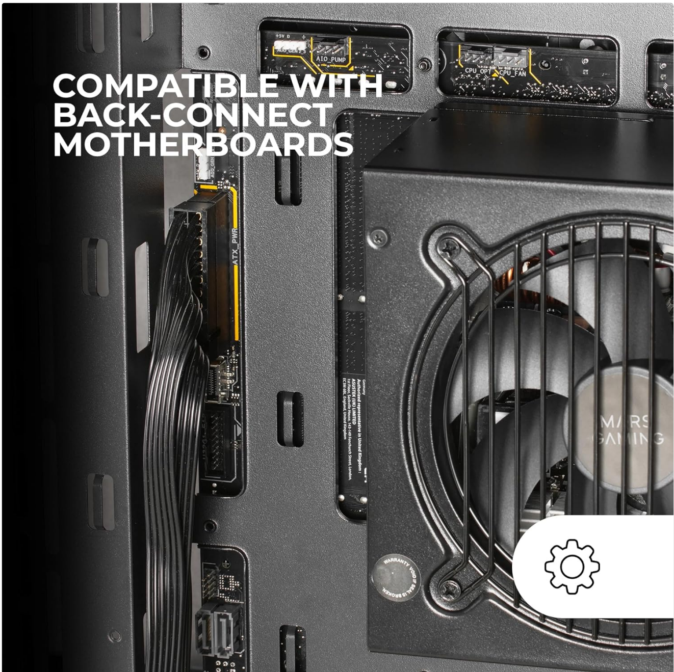
Figure 5.3: The case supports back-connect motherboards, allowing for superior cable management and a cleaner interior.
