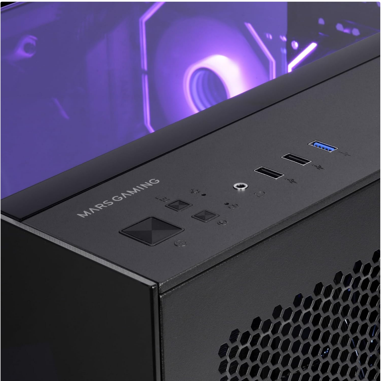
Figure 5.6: The conveniently located front I/O panel provides easy access to USB 3.0 ports and audio jacks.
