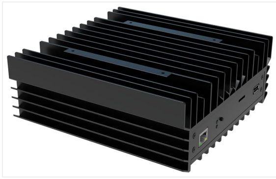
Figure 4.4: Angled view of the ICERIVER ALEO AE0 Miner, showcasing its compact form factor and robust cooling fins.
