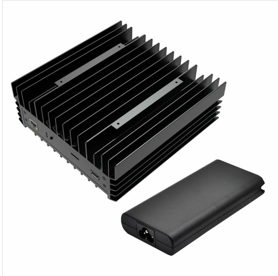
Figure 4.1: ICERIVER ALEO AE0 Miner, top-down view, showcasing the heat sink fins for thermal management.
