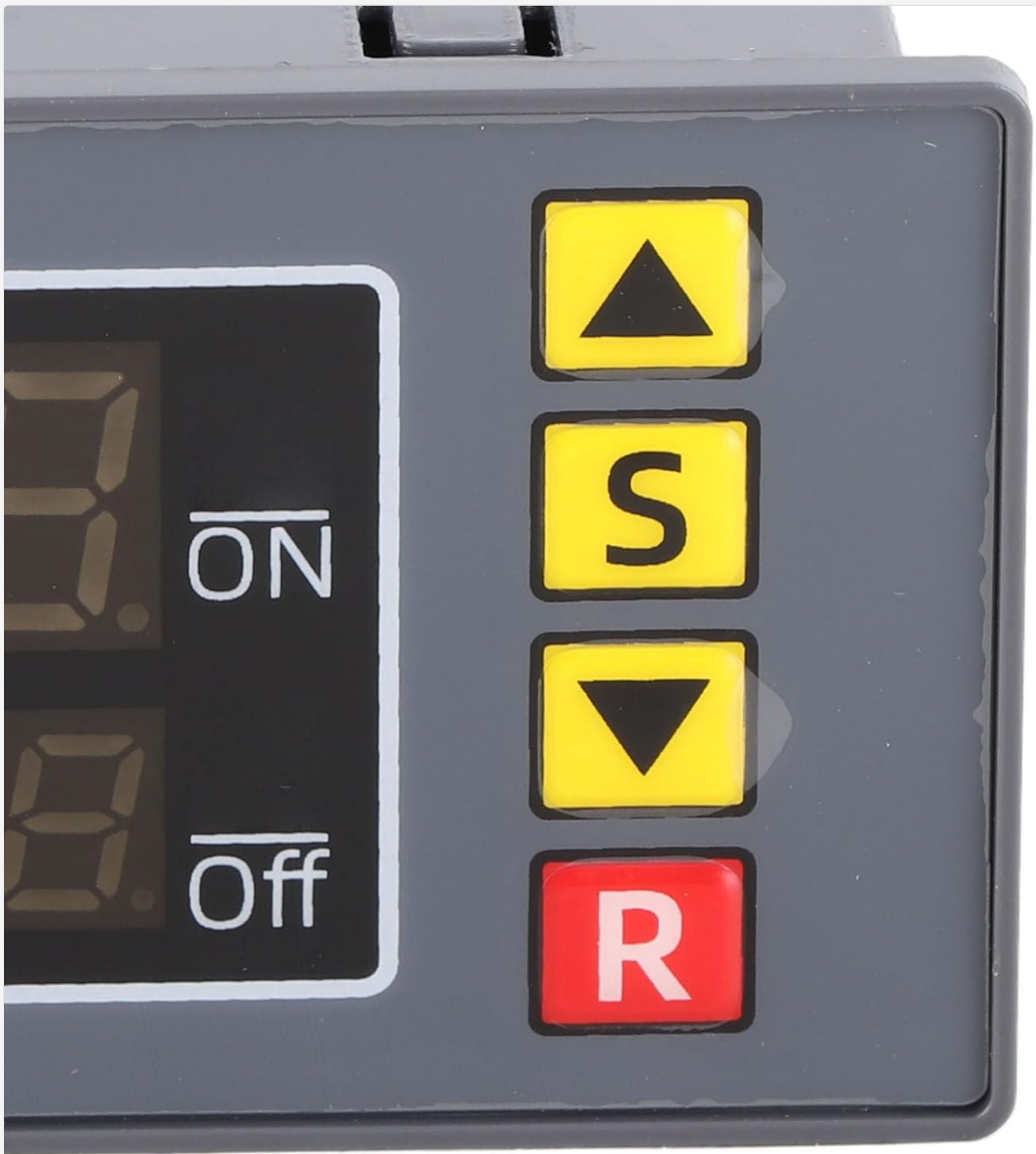
Figure 3: Detailed view of the module's front panel, highlighting the digital display for ON/OFF times and the four control buttons: UP, SET, DOWN, and RESET/RUN.
