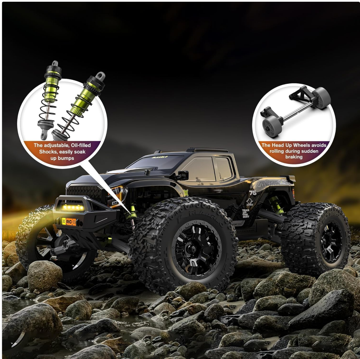
Figure 2.4: Adjustable oil-filled shocks and head-up wheels for stability.
