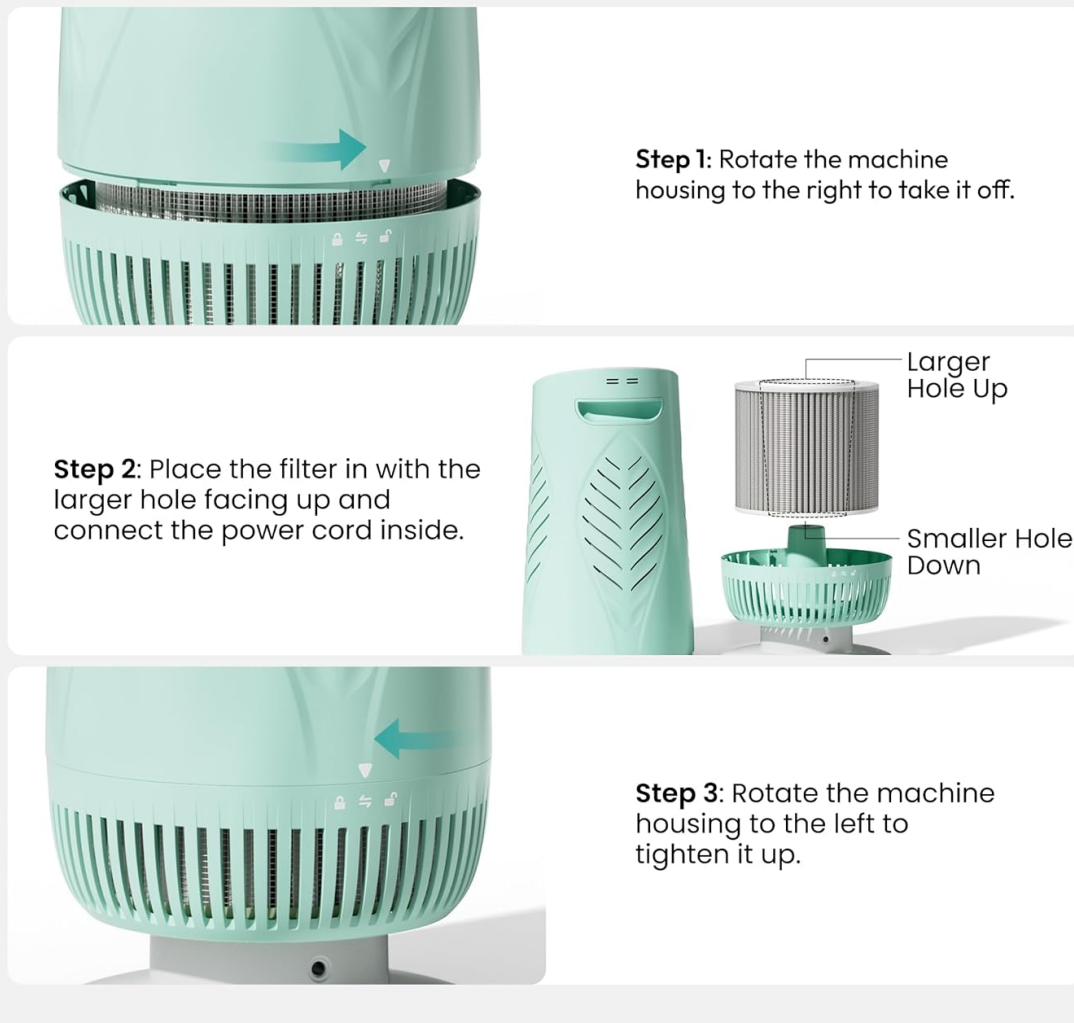
Image 2.1: Visual guide for filter replacement steps.
