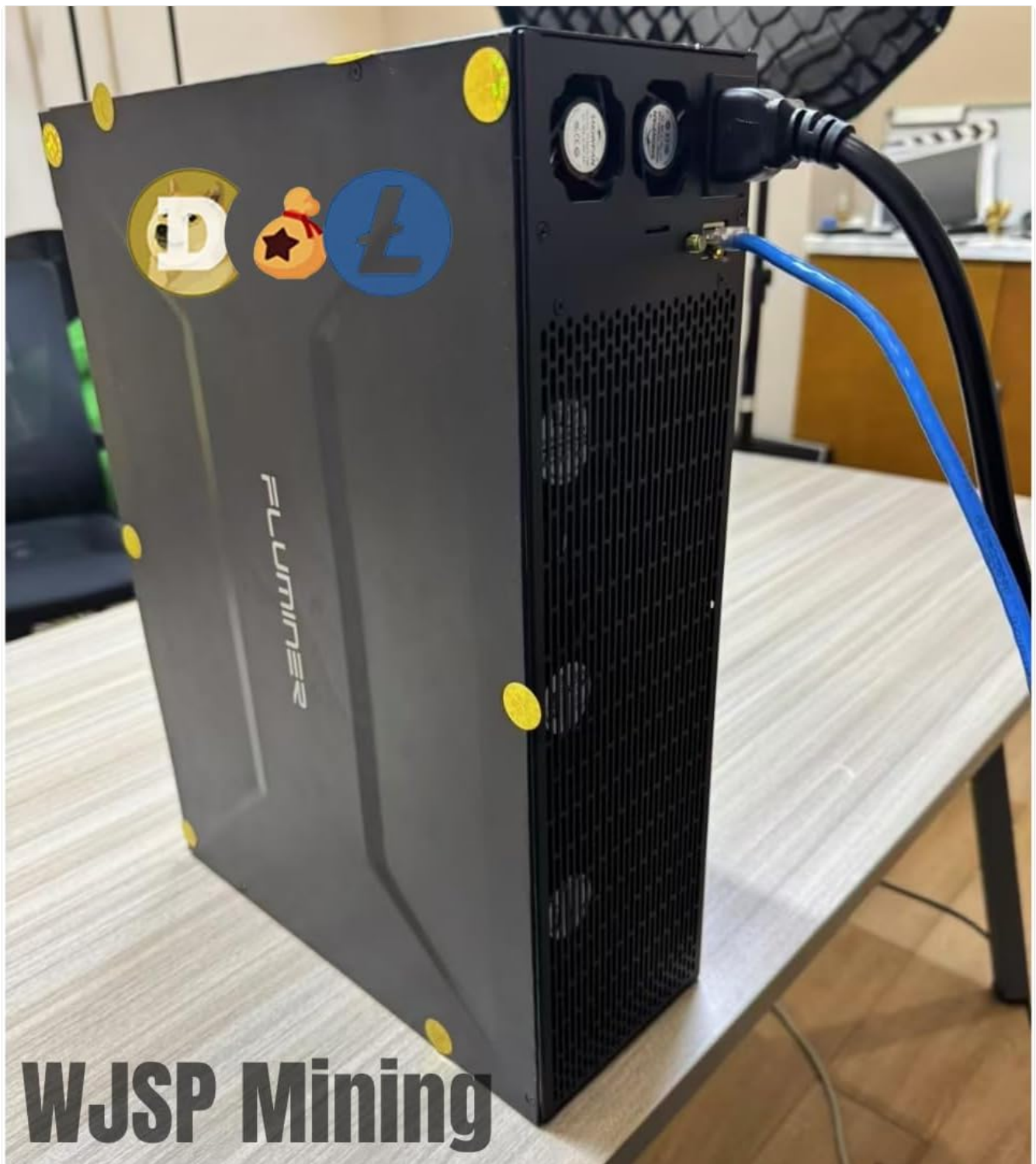
Figure 2.2: The Fluminer L1 miner with power and network cables connected, ready for operation.
