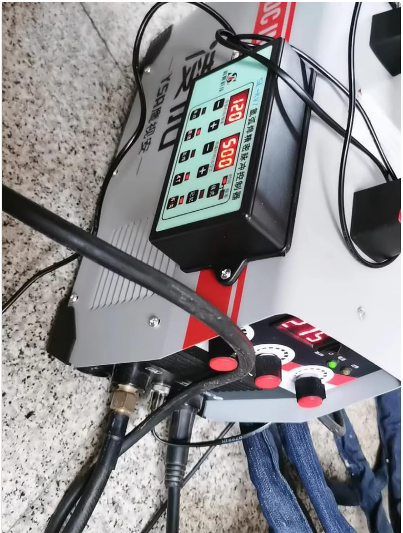
Figure 5.2: Example of the SL-KV7 controller integrated with an argon arc welding machine, showing the control cable connection.
