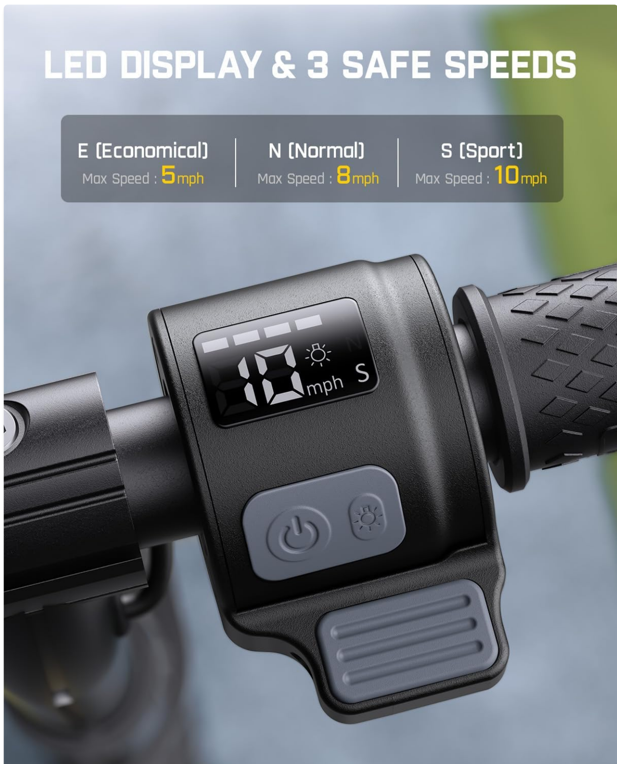
Image 5.1: Close-up of the LED display, showing battery level, current speed, and selected speed mode (E, N, or S).
