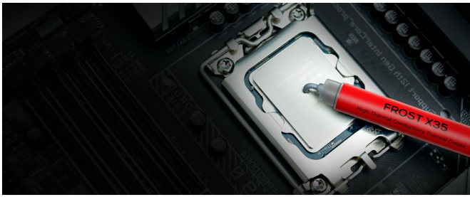
Image: Illustration of applying thermal paste to the CPU before heatsink installation.
