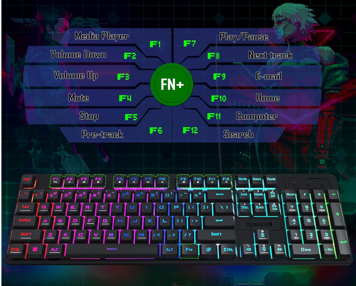
Image: The Redragon S107 Gaming Keyboard illustrating the FN key combinations for multimedia functions.
