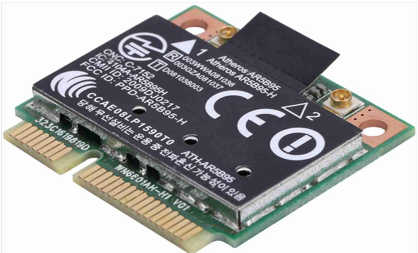
Image: Bottom view of the AR5B95 card, showing the gold-plated PCI-E contacts and a label with MAC address and other identifiers.
