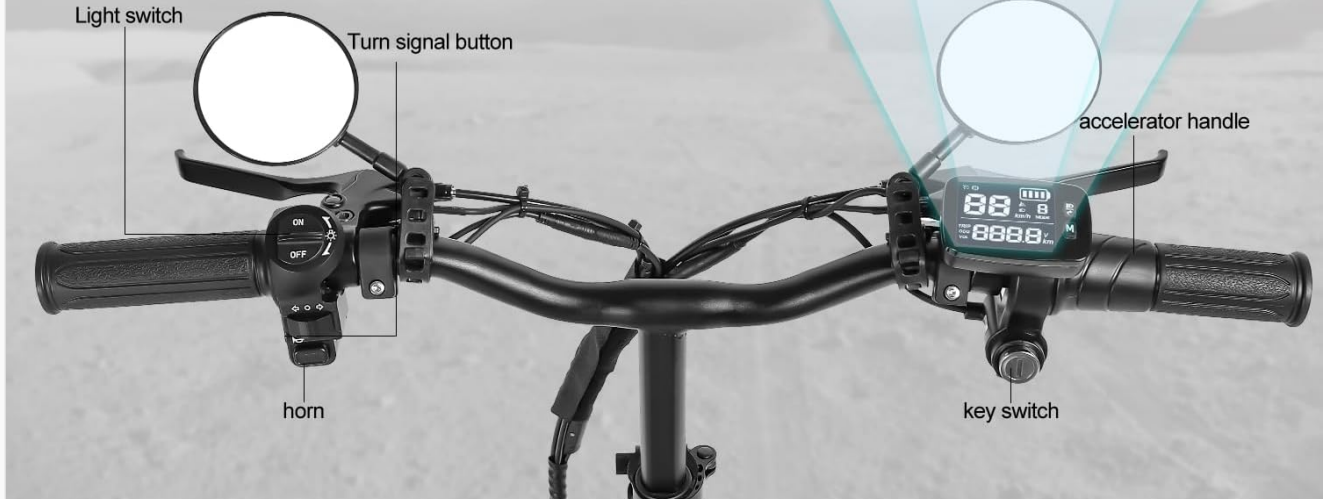
Figure 2.6: The LCD display and handlebar controls for easy operation.
