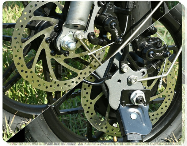
Figure 2.5: The 160mm diameter perforated brake discs provide great braking power.
