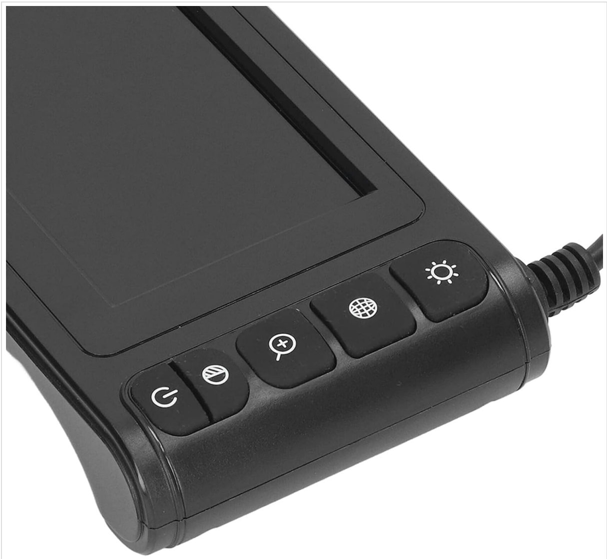
Figure 4: Control buttons on the endoscope display unit, including power, brightness, and zoom controls.
