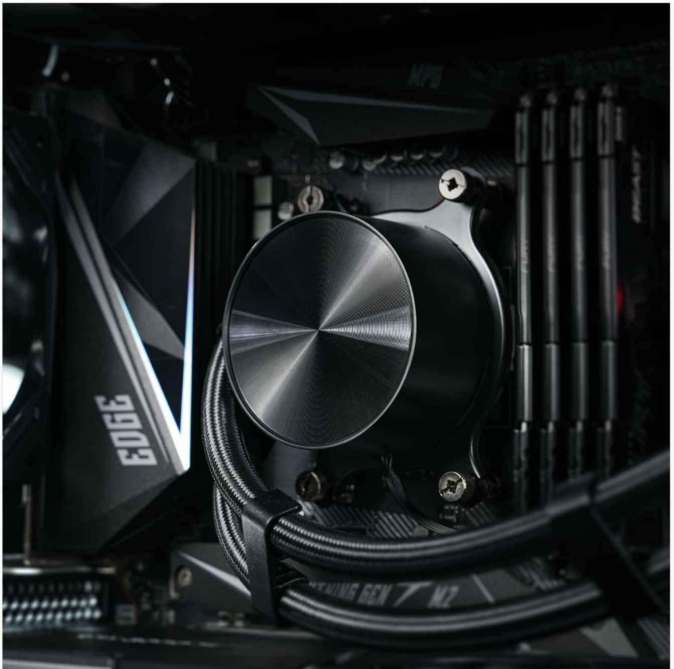
Image Description: The pump assembly mounted on the CPU, with tubes extending towards the radiator.
