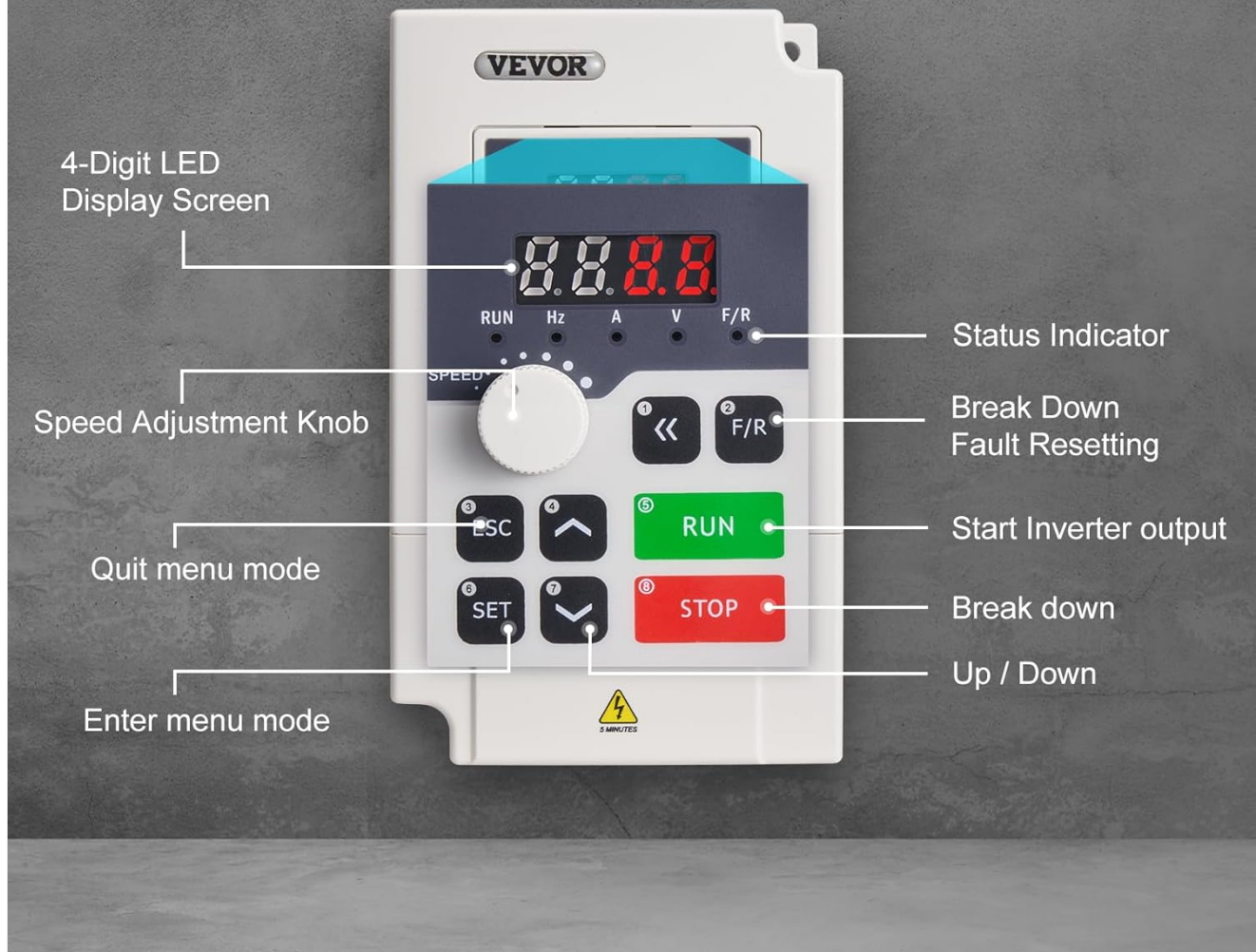
Figure 2.1: VFD Control Panel Layout. This image shows the front panel of the VFD, highlighting the 4-digit LED display, speed adjustment knob, and various control buttons including RUN, STOP, ESC, SET, and arrow keys for navigation and parameter adjustment. A status indicator is also visible.
