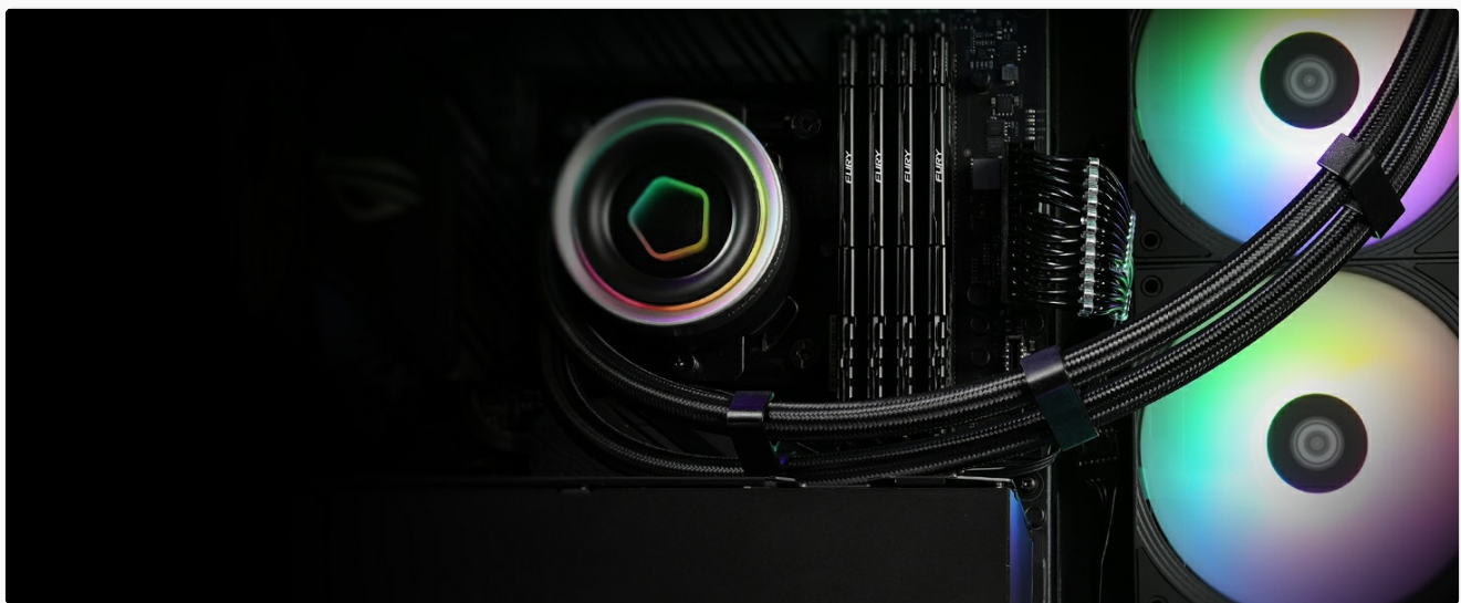
Image 2.5: The pump cap can be rotated 360 degrees for optimal orientation.
