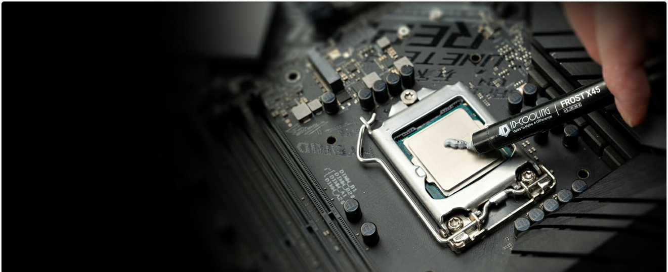
Image 4.2: Proper application of thermal paste to the CPU surface.
