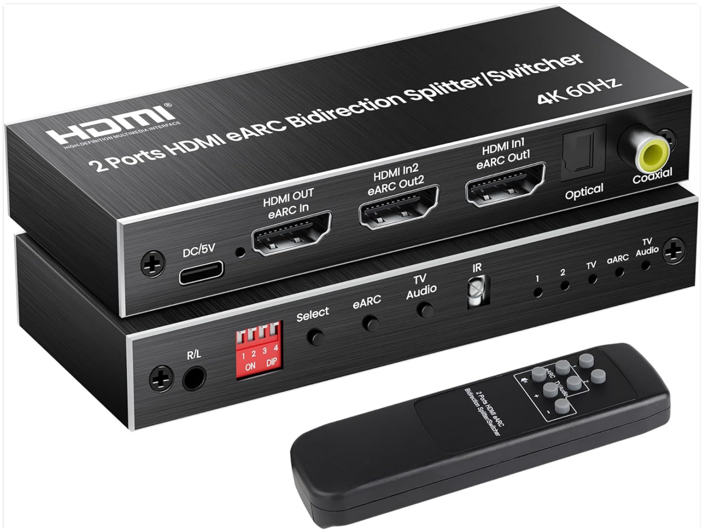
Figure 1.1: avedio links HDMI eARC Bi-Directional Switch/Splitter and included remote control.
