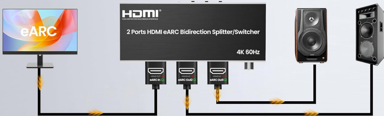
Figure 5.1: 2x1 HDMI Switch Connection Diagram.
