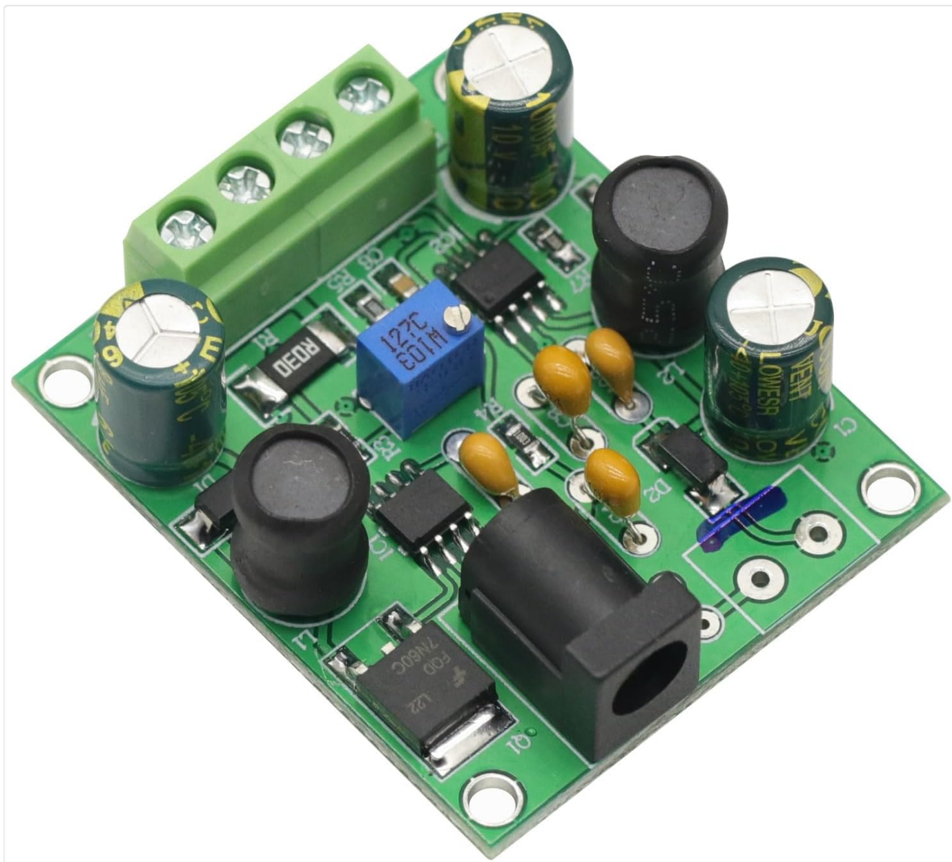
Image 1.1: Top-down view of the GODIYMODULES High Voltage DC Converter Module Board. This image shows the overall layout of the components, including capacitors, inductors, the DC input jack, and the terminal blocks for input and output connections.
