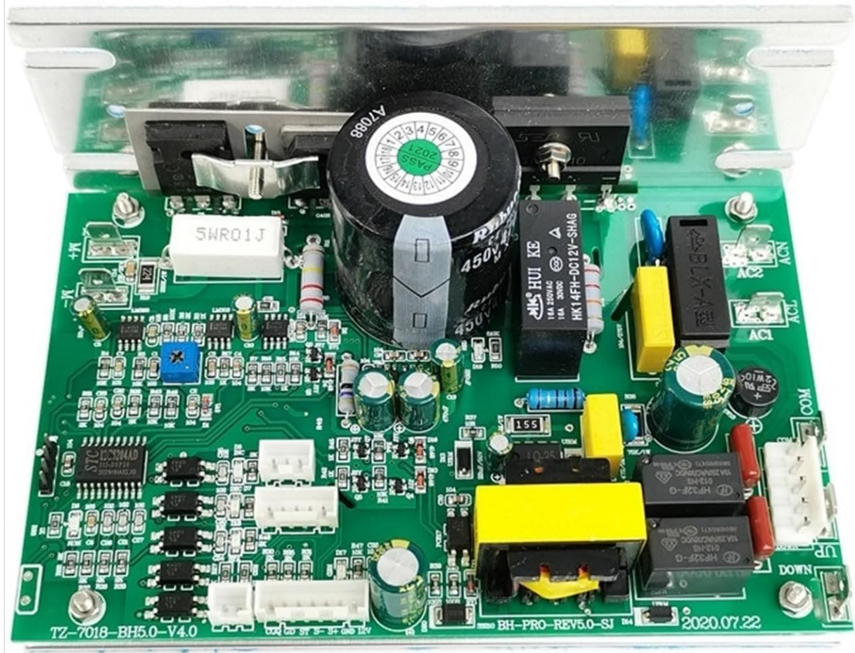
Figure 1: Top view of the DCMD76/DCMD75 Motor Controller.
