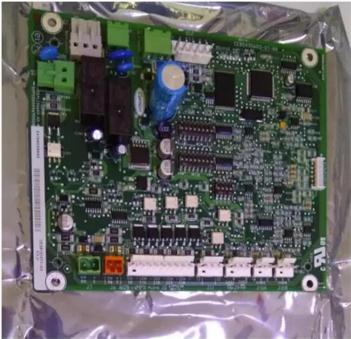
Figure 4.1: The JYFORNWC Carrier Air Conditioner Motherboard, typically shipped in anti-static packaging. This view highlights the various connection points and the overall form factor, crucial for proper alignment during installation.
