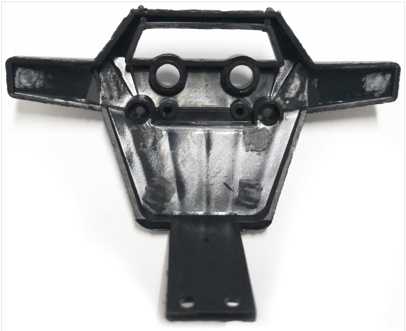
Figure 2: Rear view of the Fyfracing RC car bumper, highlighting mounting points.
