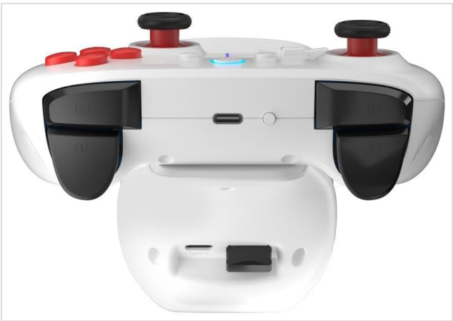
Figure 3.4: Rear view of the gamepad, detailing the placement of the LB/RB shoulder buttons, LT/RT triggers, and the USB-C charging port at the top edge.
