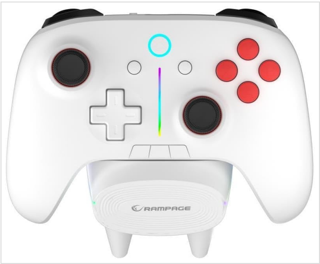
Figure 3.3: Top-down view illustrating the full button layout, including analog sticks, D-pad, action buttons, and central function buttons, with the RGB light bar visible.
