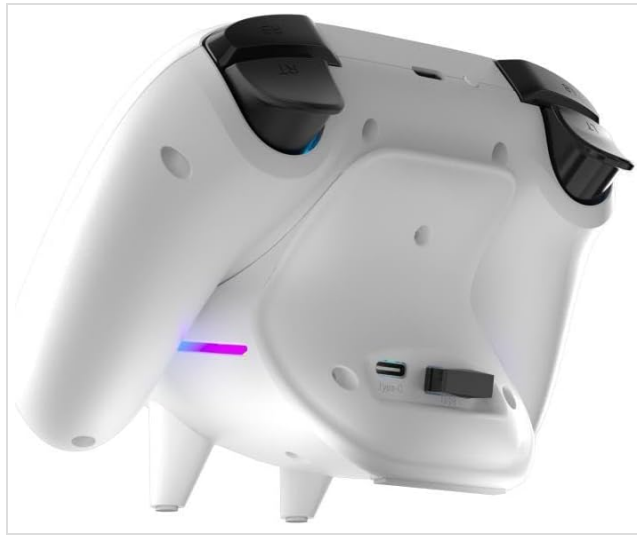
Figure 3.5: Side-rear perspective of the gamepad, providing a clearer view of the USB-C port for wired connection or direct charging.
