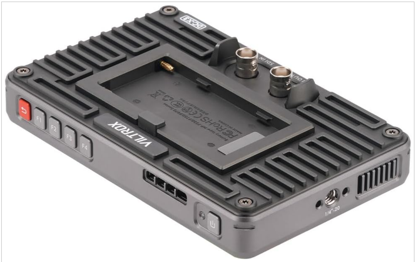
Figure 3.1: Rear view of the DC-X3, highlighting the NP-F battery plate and SDI input/output ports.
