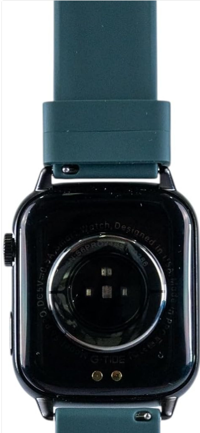
Figure 2: Rear view of the G-TIDE Smartwatch S6 Pro. This side houses the advanced optical sensors for heart rate and blood oxygen monitoring, along with the magnetic charging contacts. Product information and certifications are also visible.
