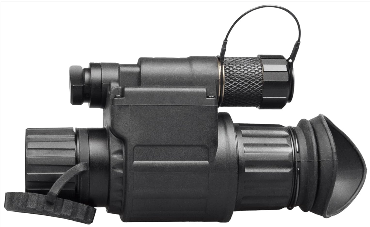
Figure 4: Side view of the Wolf-14 monocular, indicating the IR illuminator and control knob positions.
