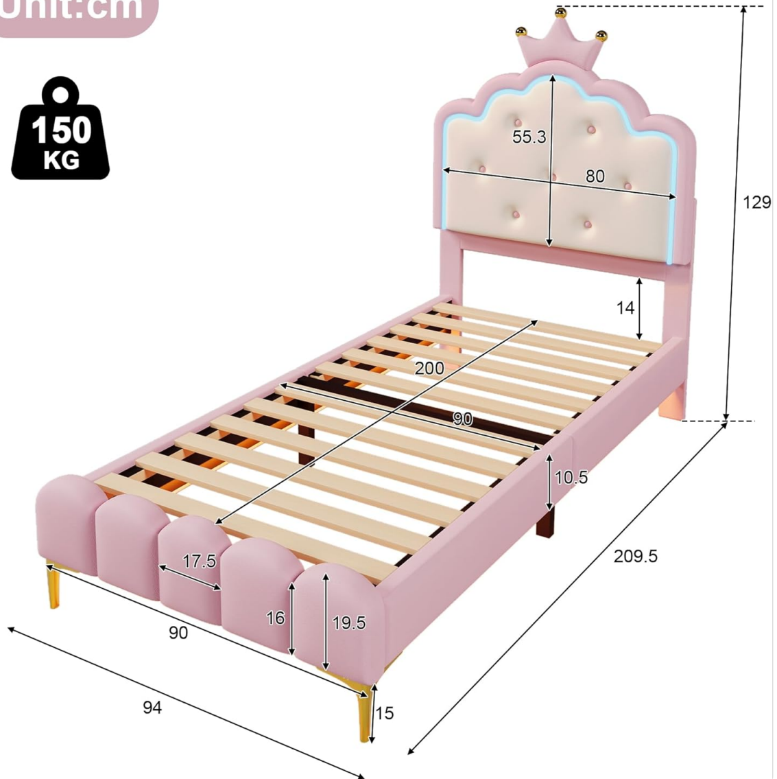
Figure 3.1: Product dimensions and key components. This diagram illustrates the overall size and individual parts of the bed, including the headboard, footboard, and slatted frame, with measurements in centimeters.
