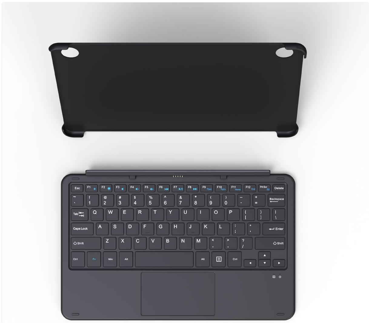
Figure 2.1: An overhead view of the Zwide G105U docking keyboard with an integrated touchpad, shown alongside its protective case. The keyboard features a standard QWERTY layout with function keys, media controls, and a Windows key. The protective case is designed to hold a tablet and can function as a stand.
