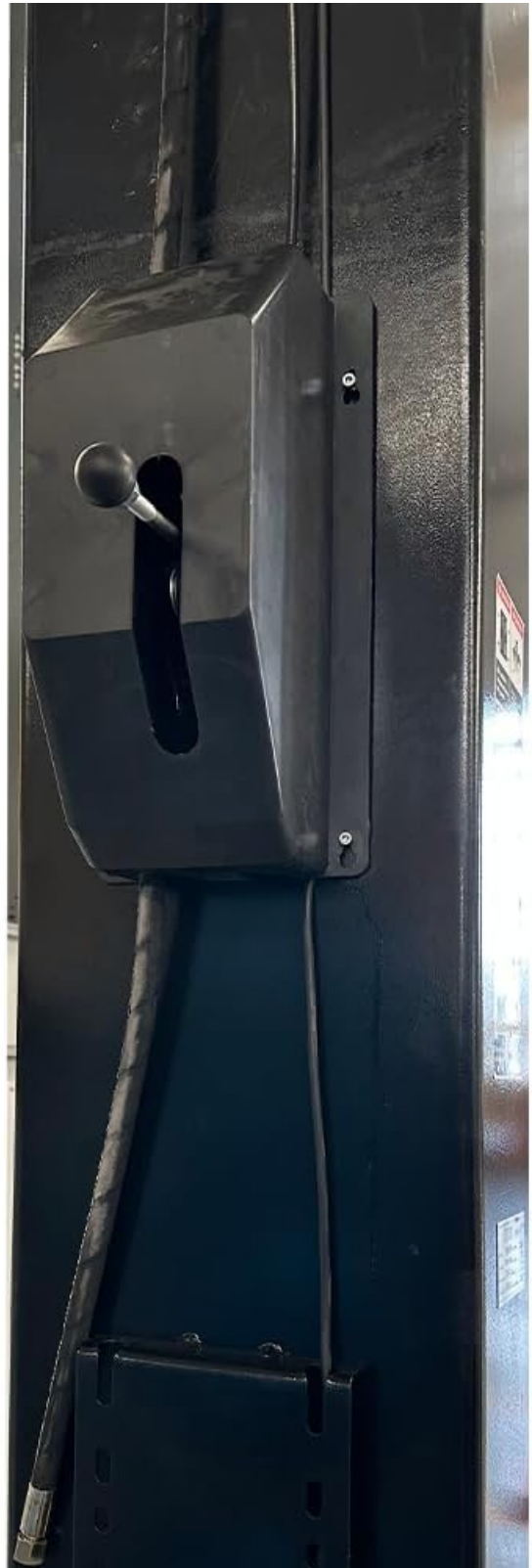
Figure 3.3: Single Point Lock Release. This image displays the single point lock release lever, which allows for convenient and secure disengagement of all safety locks from one location.
