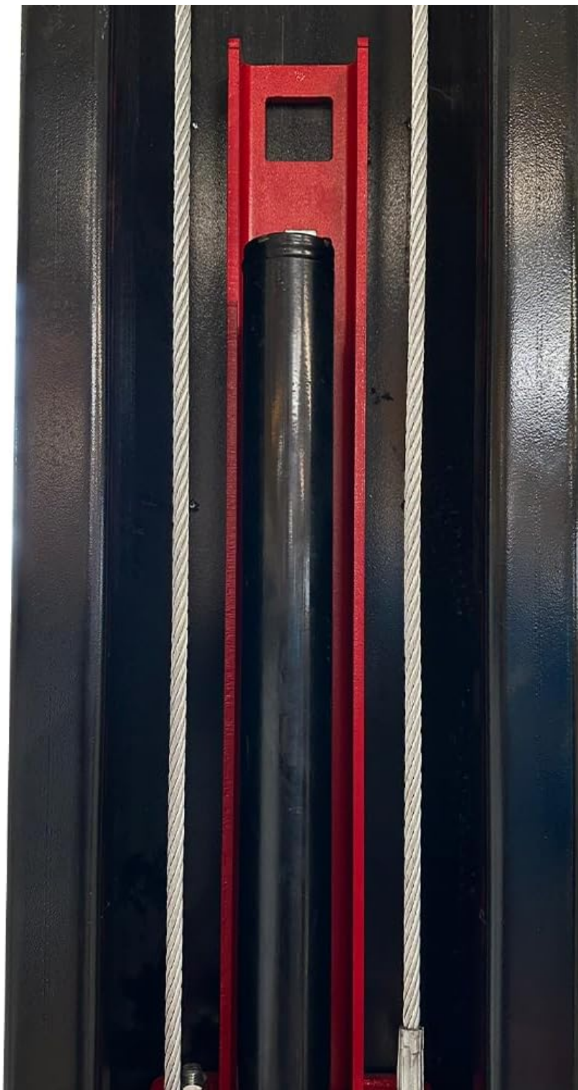
Figure 3.5: Cylinder Direct Drive. This image shows the hydraulic cylinder and chain-drive system, illustrating the direct drive mechanism responsible for the lift's powerful and reliable operation.
