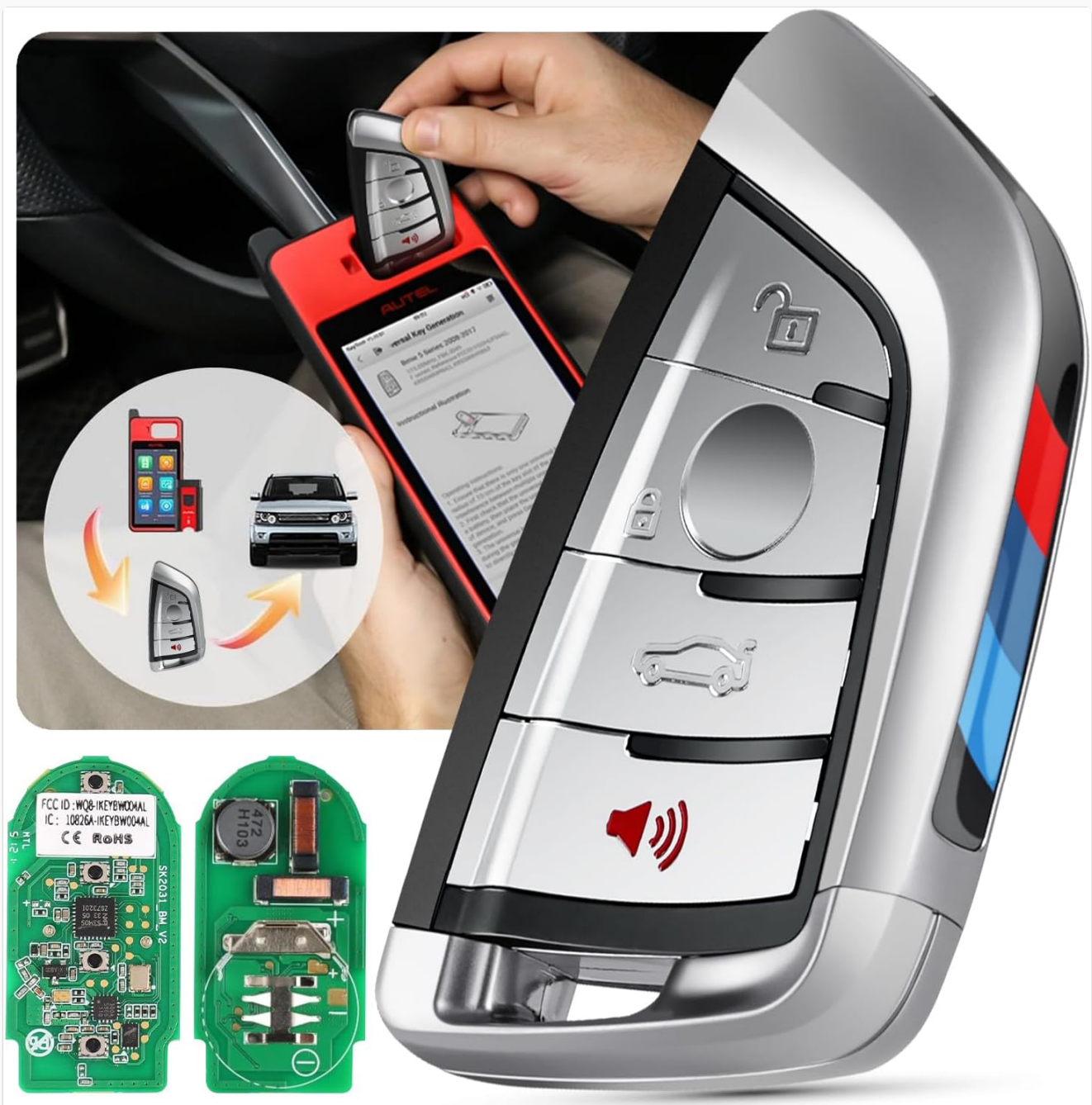
Figure 5.1: Key Fob Programming. This image shows the Autel IKEYBW004AL key fob being placed into an Autel programming device, ready for the generation process.
