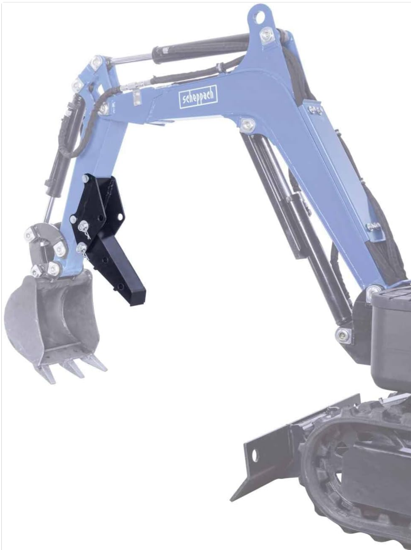
Image 1: The Scheppach Excavator Thumb Attachment mounted on a Scheppach Mini-Excavator EXC815, demonstrating its integrated position for gripping.
