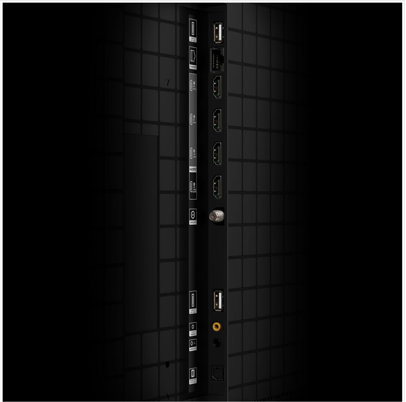
Close-up view of the rear input/output ports on the TCL 98X11K TV, including multiple HDMI and USB ports, and an antenna input.
