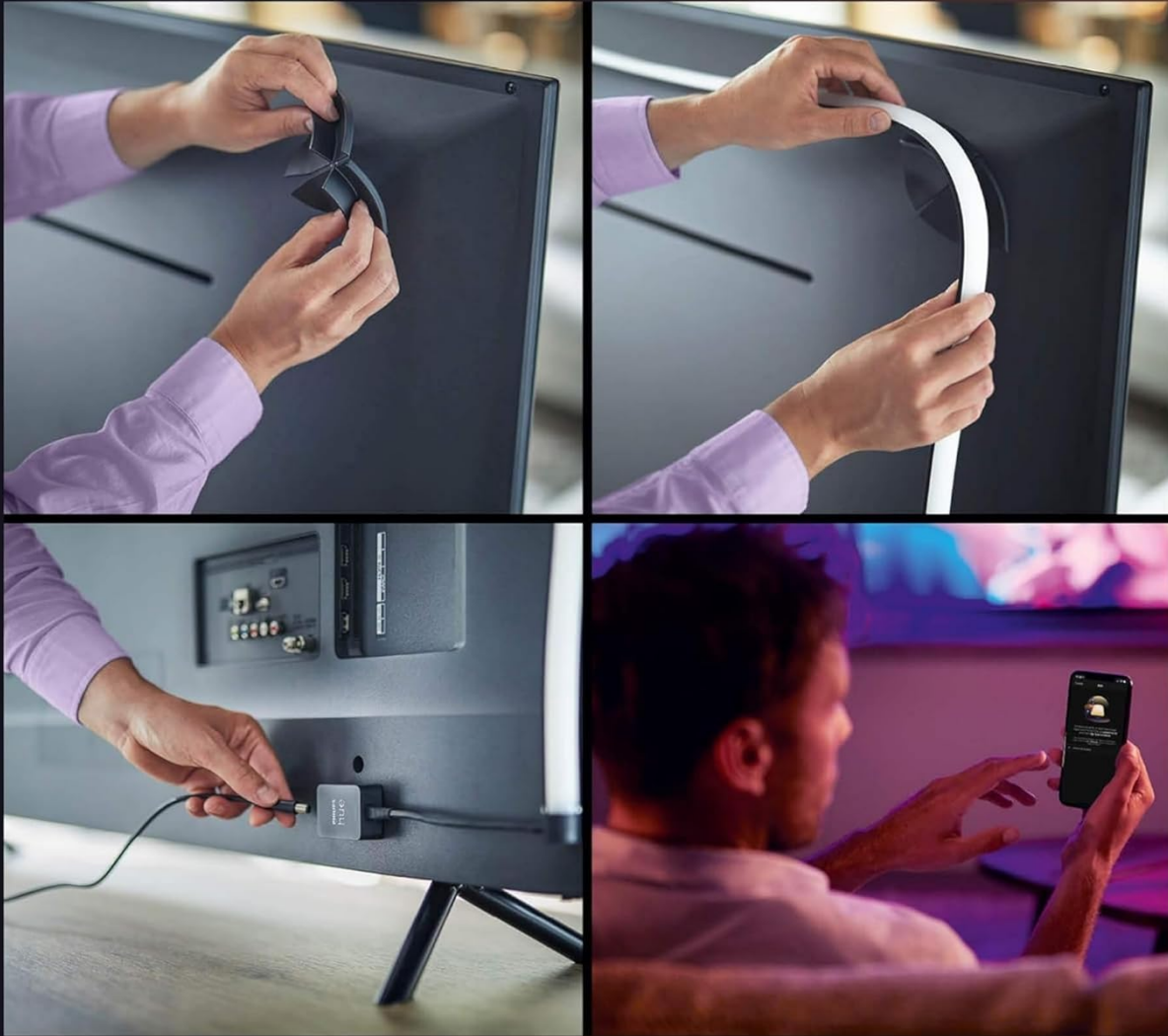
Image: Visual guide for installing the light strip and connecting the sync box.
