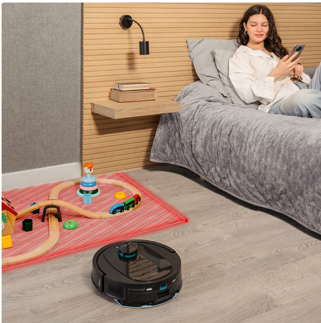
Image 6.2: The robot demonstrating its ability to avoid a designated restricted area, indicated by a red overlay,
