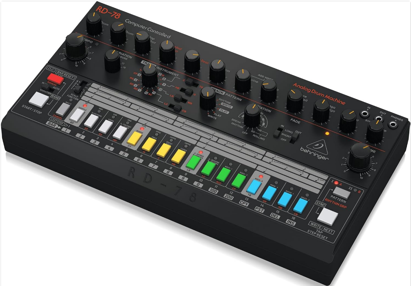
Figure 4: Close-up angled view of the RD-78. This image focuses on the variation, fade, and volume controls, essential for dynamic performance.
