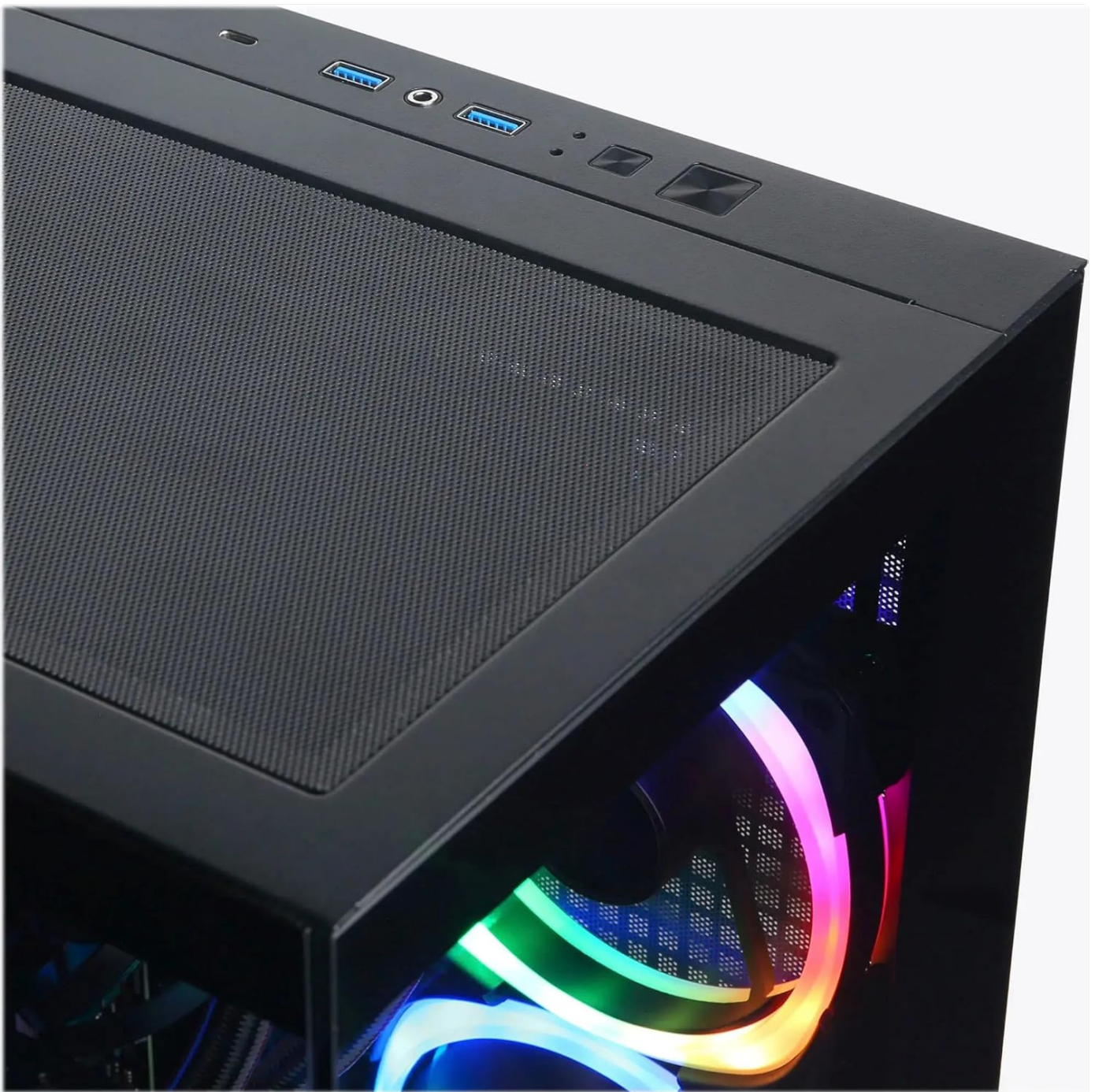
Image: Top I/O panel with USB ports, audio jacks, and power button.
