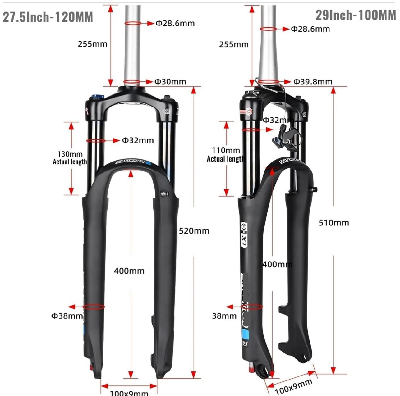
Image: Dimensional diagram of the suspension fork. This illustration provides detailed measurements for both 27.5-inch (120mm travel) and 29-inch (100mm travel) fork models, including steerer tube length, stanchion diameter, and axle spacing.
