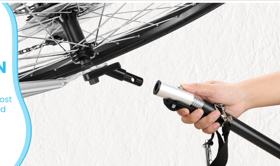
Image 4.1: Illustration of the easy installation process, showing the universal coupler being connected to a bicycle's rear axle.
