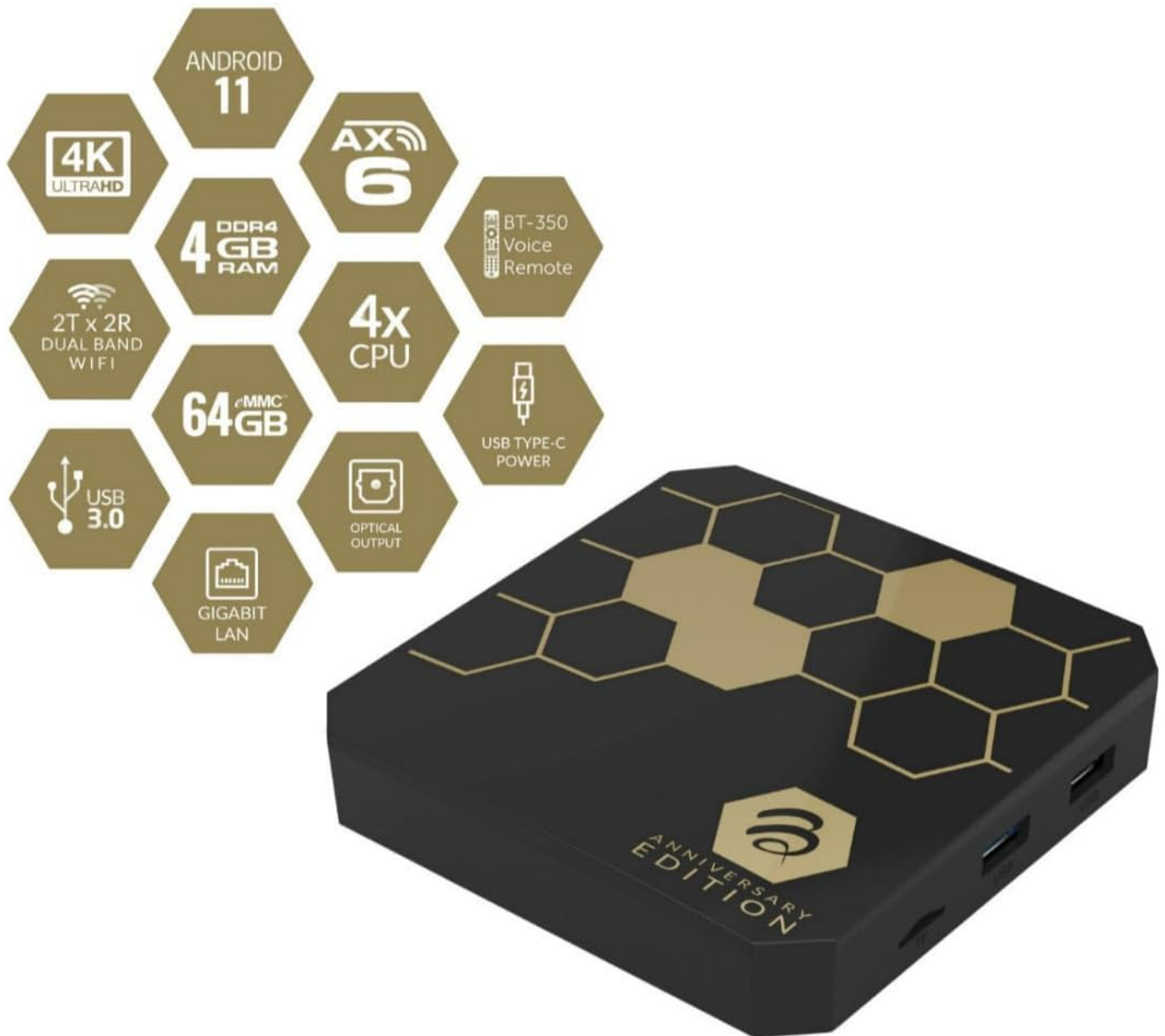
Image: The BuzzTV Classic Anniversary Edition device with graphical callouts indicating its key features, including 4K UHD, Android 11, AX6 Wi-Fi, 4GB DDR4 RAM, 4x CPU, BT-350 Voice Remote, 2T x 2R Dual Band Wi-Fi, 64GB eMMC storage, USB Type-C Power, USB 3.0, Optical Output, and Gigabit LAN.
