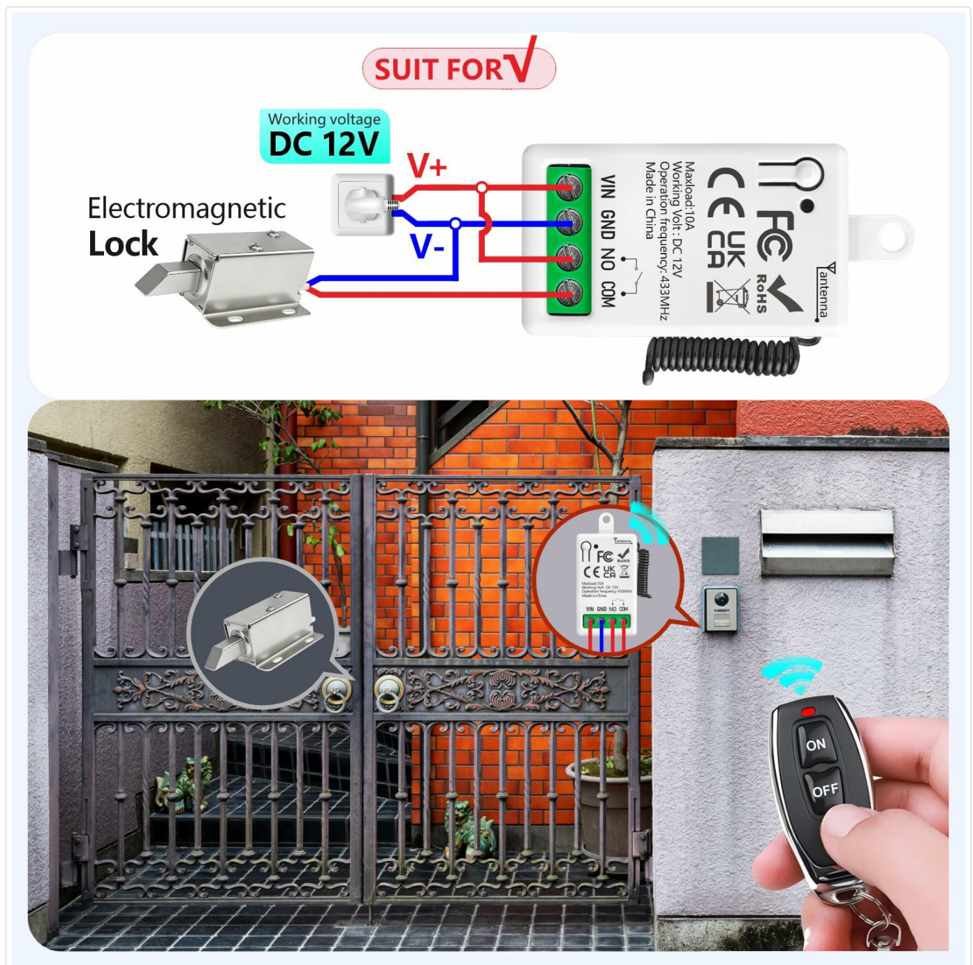
Figure 6: Electromagnetic Lock Wiring
