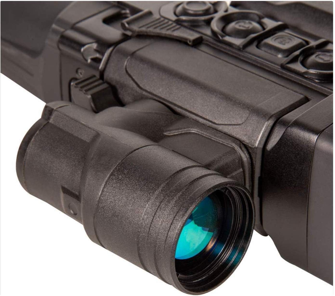
Figure 4.2: Close-up of the detachable IR illuminator
