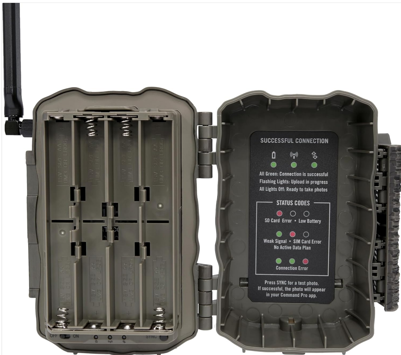
Internal view of the camera, showing the battery tray and connection status indicators for easy setup and troubleshooting.
