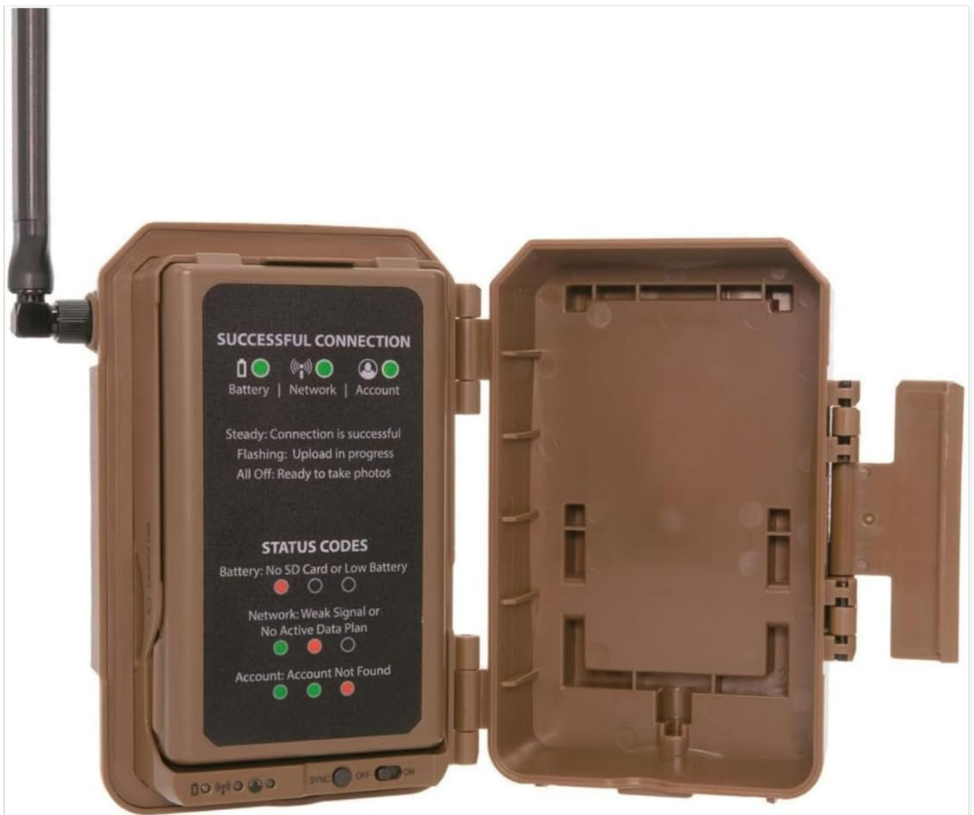
Figure 2: Internal view of the camera, highlighting the battery tray and status indicators.
