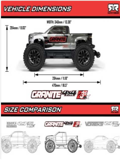
Image: Diagram illustrating the key dimensions of the ARRMA Granite 4X4 3S BLX Monster Truck.
