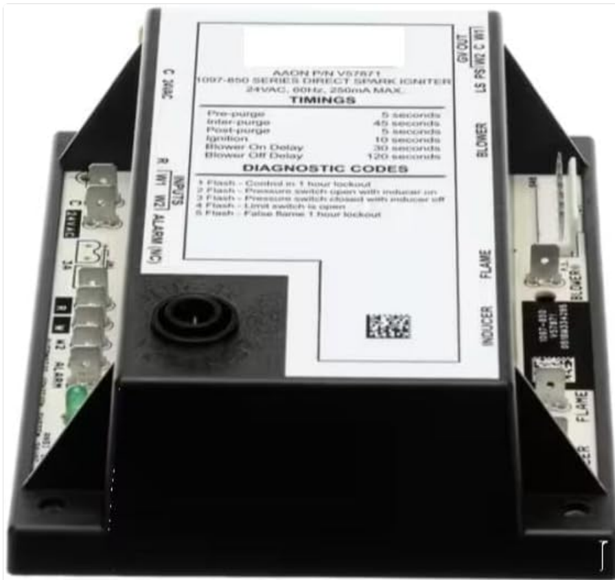
Figure 1: AAON 1097-850 Ignition Module. This image displays the top view of the ignition module, highlighting the product label with detailed timings for various operational stages (Pre-purge, Inter-purge, Post-purge, Ignition, Blower On Delay, Blower Off Delay) and a list of diagnostic flash codes. Various electrical connection terminals are visible on the sides, labeled for inputs and outputs such as 24VAC, GV OUT, LS PS W2 C W1, Blower, Flame, Inducer, and Alarm (NC).
