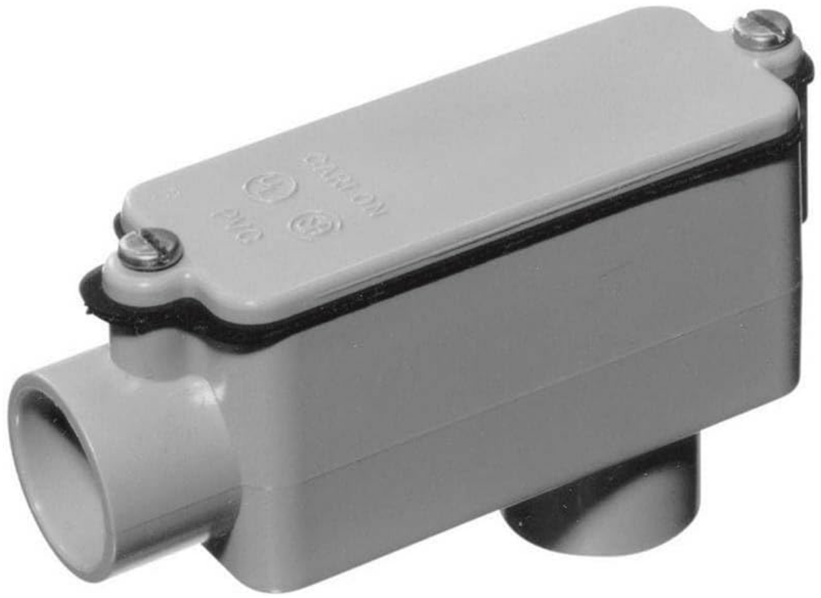
Image 1: Carlon E986E-CTN Type LB Conduit Body. This image displays the gray PVC conduit body with its removable cover, showing the 3/4 inch opening for conduit connection and the 'LB' shape for a 90-degree turn with rear access.
