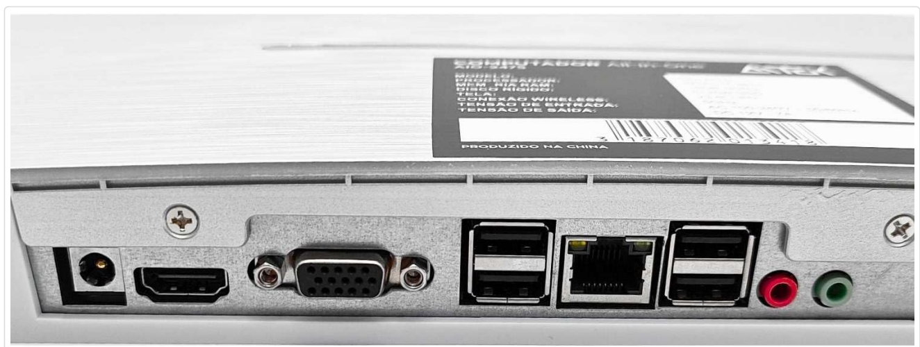
Image 4.5: Detailed view of the rear connectivity ports, including power input, HDMI, VGA, USB, Ethernet, and audio jacks.
