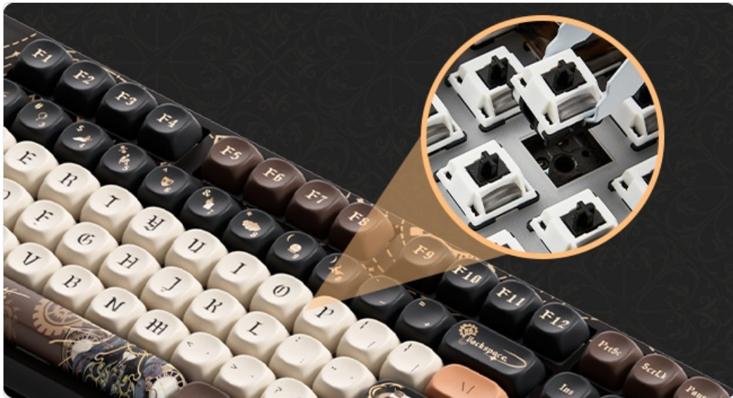
Figure 5: Detailed view of a switch being removed from the keyboard socket.
